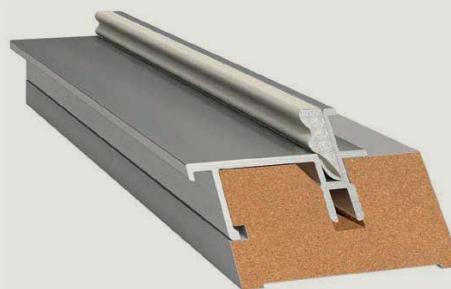
Constructive Solution For a Jamb
